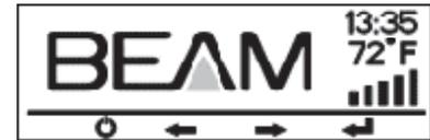
The flashing Main Screen indicates that the power unit has automatically recovered from an error situation and will operate properly when powered on.
